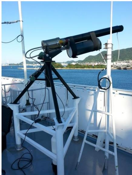
Photo shows Buccaneer muzzle loaded with underslung payload as well as a remote firing cable (pictured at the rear of the mount).
